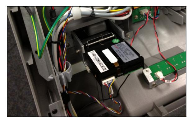
When you install the new card reader, we recommend leaving the screws a little loose, and then try inserting a card in from the front. The card should slide in and out easily without hanging up on the bezel.
