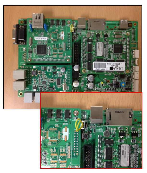
Once the jumper has been installed, you're ready to reinstall the cover over the motherboard and verify that all the wires are attached properly.
