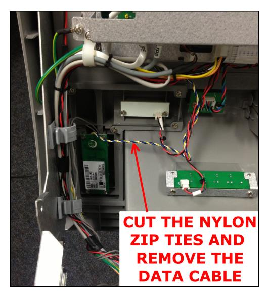
Once the cable is freed up, remove it from the ATM completely along with the card reader.
