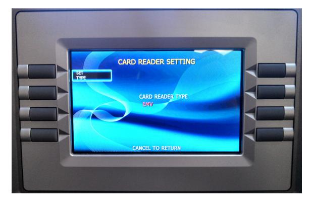
Once this has been set, return the ATM to normal operation and dip your card and remove to test and verify that it's operating normally.
