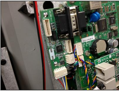
Plug the jumper wire in as shown above, the wires will be tight, so route them down under the modem so they do not get pinched. Attach the card reader wire to the bottom.
